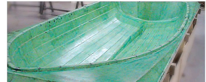
The GRP pattern is treated with ALWA RELEASE LACQUER.
